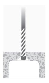
Drill a hole through the concrete into the core using a masonry bit of the correct diameter and tolerance.
