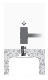
Insert cone end and tap until anchor is flush to the concrete surface.
