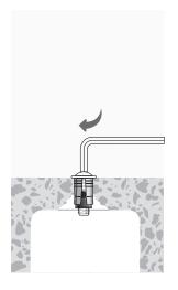
Attach setting tool or bolt and washer onto anchor and expand it by turning the hollow setting tool or bolt 3 to 4 turns or until snug.
